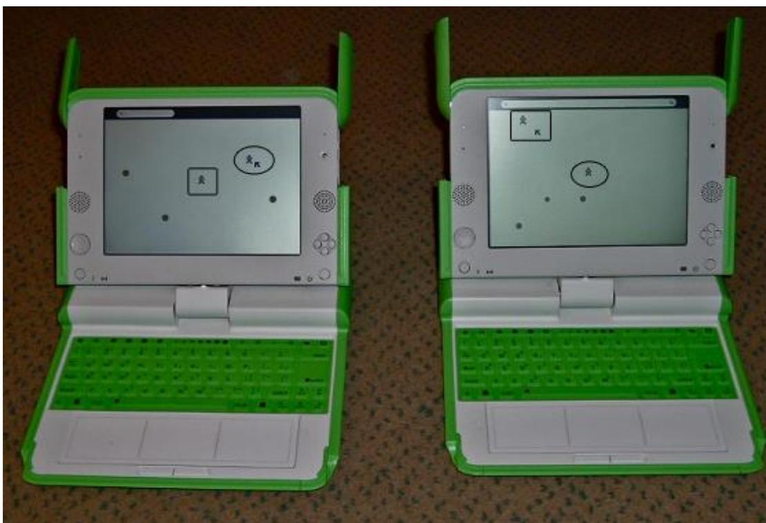
Figure 4: This edited photo shows two XO's linked in a wireless mesh network.
